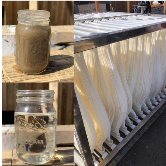
nrPUR™ Ultrafiltration (UF) Membranes consistently deliver reuse quality effluent.
